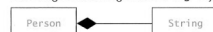
FIGURE A.10 UML Diagram Showing That String Objects Are Components of Class Person
